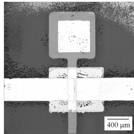
FIG. 3. Optical micrograph of an *a*-Si TFT fabricated by letterpress printed etch masks. The transistor channel length and width are  $20 \mu\text{m}$  and  $400 \mu\text{m}$ , respectively. The gate width is  $170 \mu\text{m}$ .
