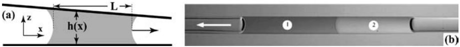
Figure 4 (a) A liquid plug with \theta < 90^\circ ( \theta > 90^\circ ) moves toward (away from) the narrow gap region. (b) A self-propelled bislug ( \gamma_{12} = 18.0 mN/m) of ethylene glycol ( \gamma_1 = 47.7 mN/m) and silicone oil ( \gamma_2 = 20.3 mN/m) in a 1 mm diameter glass capillary. [Reprinted from Bico & Quéré (2002) with permission from Cambridge Univ. Press.]
