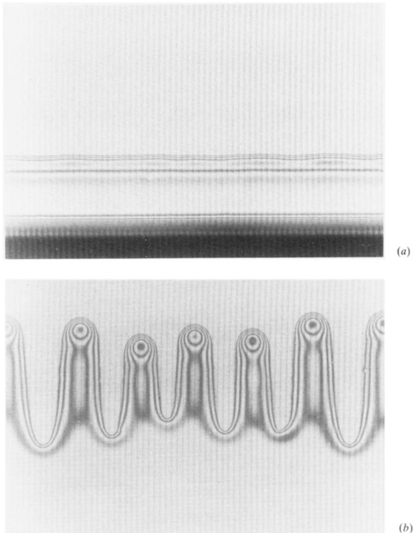
**Figure 2.** Time development (a) after 5 min and (b) after 25 min of the fingering instability at the vertically ascending front of a PDMS oil film of viscosity 20 mPa s and  $\tau = 0.18$  Pa observed under laser illumination. Measured from finger tip to tip, the wavelength  $\Lambda$  in (b) is 0.48 mm.
