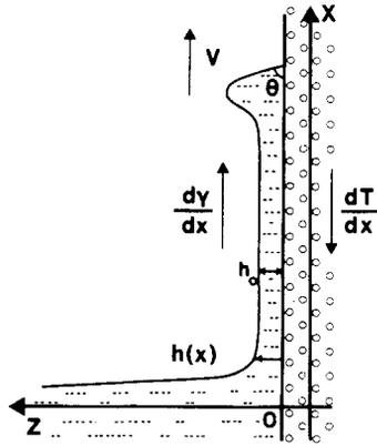
**Figure 1.** A schematic view of the capillary rise geometry in which a film of PDMS is made to climb under a gradient in surface tension. The macroscopic dynamic contact angle, measured from the reconstructed profiles and listed in table 1, is denoted by  $\theta$ .
