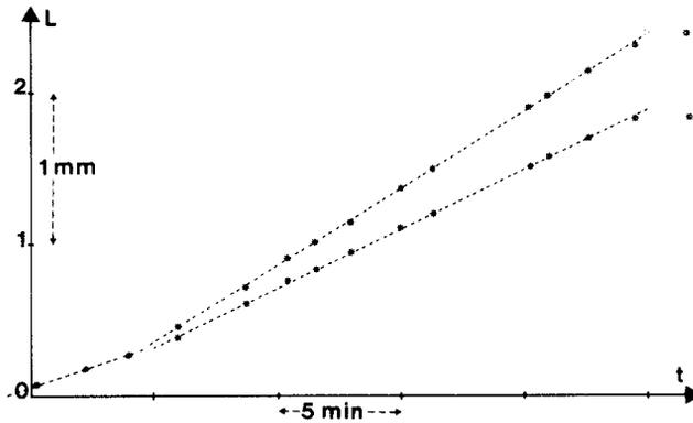
**Figure 3.** Position of the fluid front as a function of time for PDMS of viscosity 20 mPa s and  $\tau = 0.10$  Pa. The values  $V$  in table 1 are determined from the slope of the linear regime occurring before the onset of the instability.
