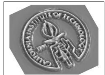
Simulation of Caltech logo formed in a 100 nm polymer film by thermocapillary patterning.
